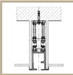
Single shielding, installation below concrete lintel
