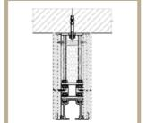
Single shielding and track casing
