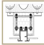
Hollow ceiling with mounting track and single shielding
