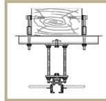
Lateral to wooden beam with mounting tracks
