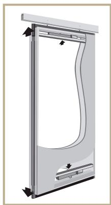
Microprocessorcontrolled lifting motors for automated panel opening and closing.
