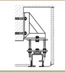
Installation with corbel, right hand: U section with track casing, left hand: L section
