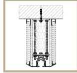
U section single shielding with track casing
