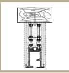
Wooden beam, single shielding with track casing
