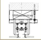
C section, double shielding with Mounting track
