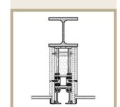
double shielding at steel girder, welded
